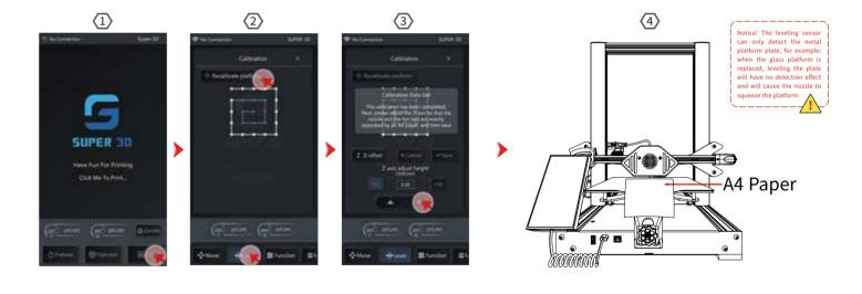
3 After the leveling is completed, begin the nozzle offset calibration. Please place a piece of A4 paper between the print head and the platform, adjust the gap between the print head and the platform by clicking [Up] and [Down], and keep push and pull the A4 paper, and compensation leveling can be completed when friction is generated.
